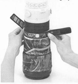
5. Wrap the focus ring with ⑤, and adhere the Velcro tightly.
